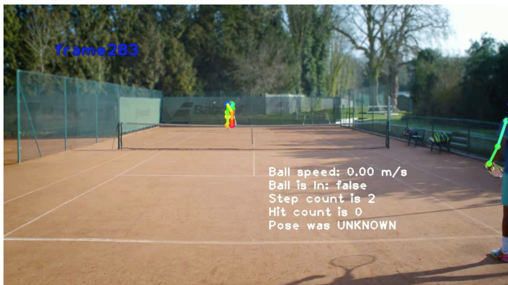
FIGURE 4.4: The image shows the unanticipated labels for the player on the far side of the court. In addition, the player close to the camera does not have a full skeleton due to not showing the full body.
