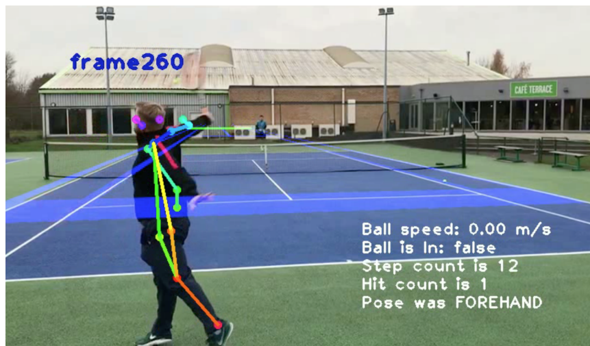
FIGURE 4.5: The image shows the unanticipated labels for the player when standing sideways. As one may see, the coordinates of legs overlap with each other.
