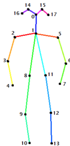
FIGURE 4.3: The skeleton labels that would be drawn on the detected human. Each joint is mapped to a unique number. For example, head is mapped to 0 and left shoulder is mapped to 2.
